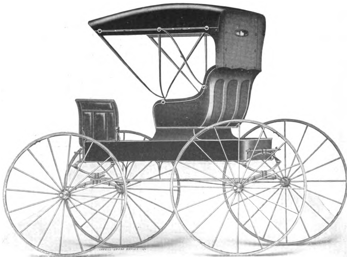
TRIPLE PANEL AUTO SEAT BUGGY Built by W. A. Paterson Co., Flint, Mich.
